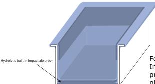
Features that provide additional protection include an Interphase Protector (sacrificial layer), and impact protection such as hydrolytic bottom and impact plates.
